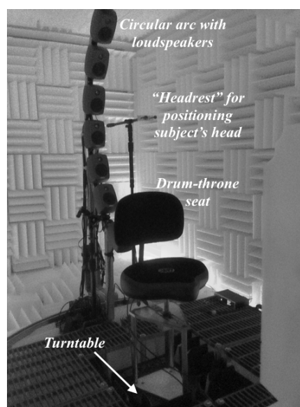
Fig. 1: Setup used to make HRTF measurements.
